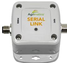
Mount the Serial Link device to the front of the grain cart with its connectors pointing sideways, preferably protected from direct exposure to the elements. Connect the Serial Link 12-volt power cable to the device.
